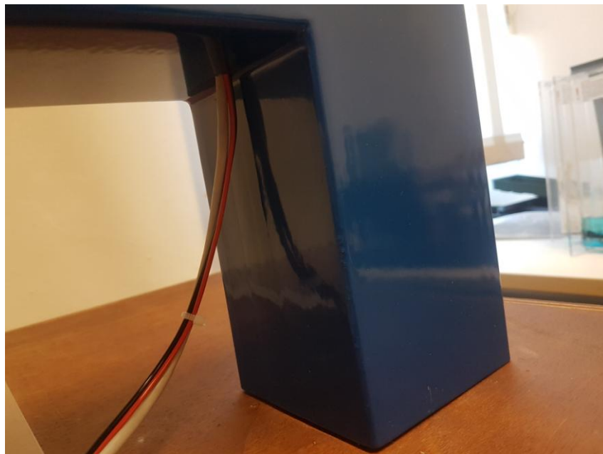
Figure 3.5. Hole for wires from actuator and solenoid
