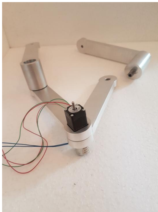
Figure 2.22. All four links assembled with bearings, actuator and solenoid
