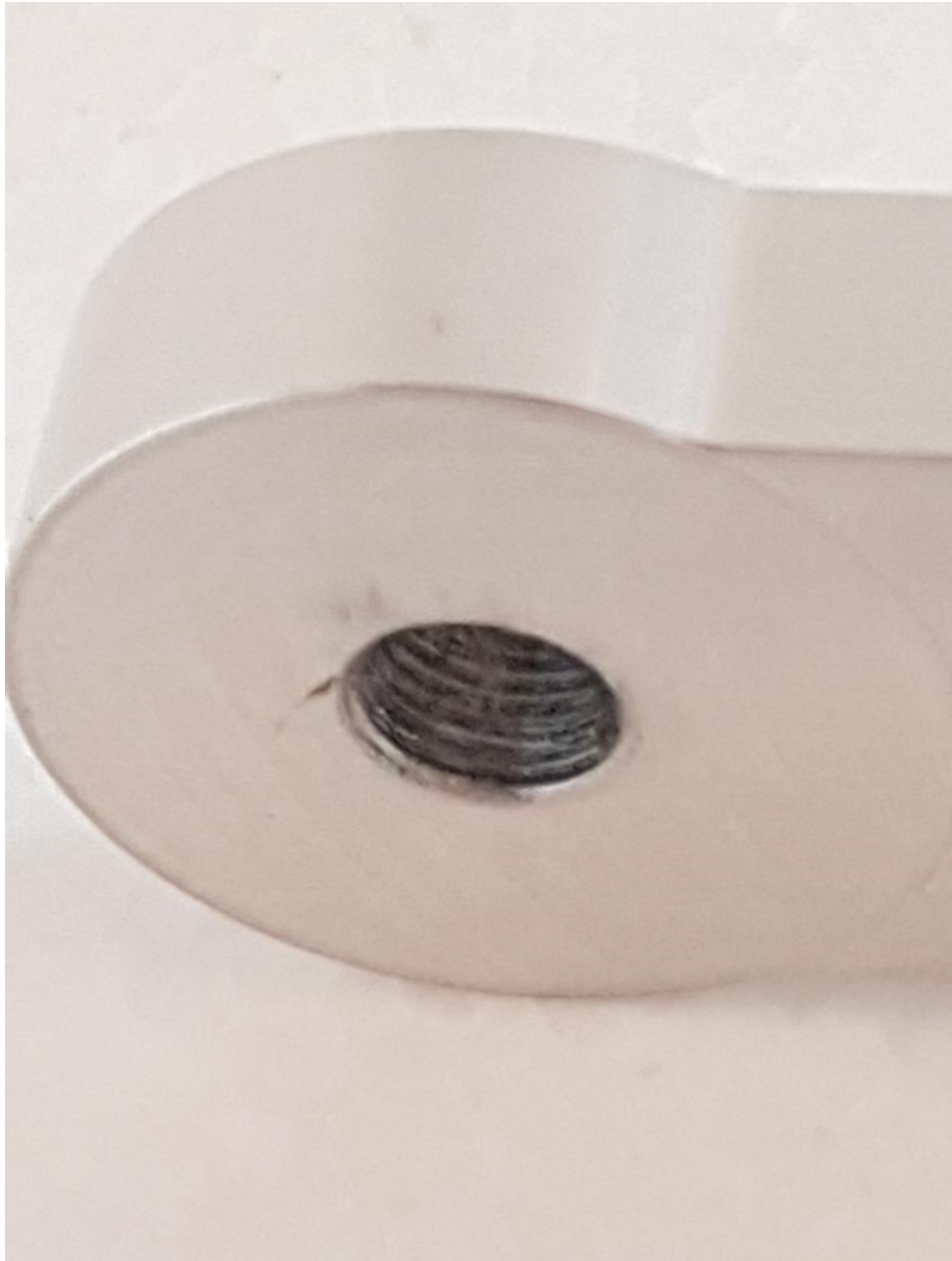
Figure 2.18. Thread on secondary arm where type 2 bearing can be screwed in to
