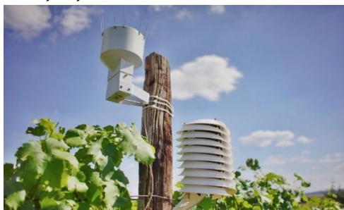
Slika 5. allMETEO senzor Izvor: Eastern Peak, 2022.
