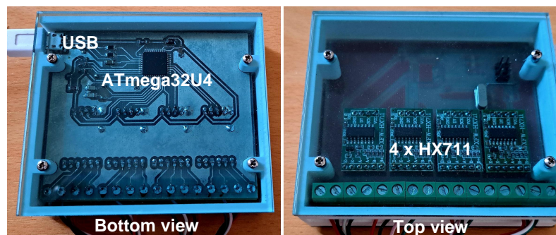
Figure 9. Electronic board for measuring and PC communication.
