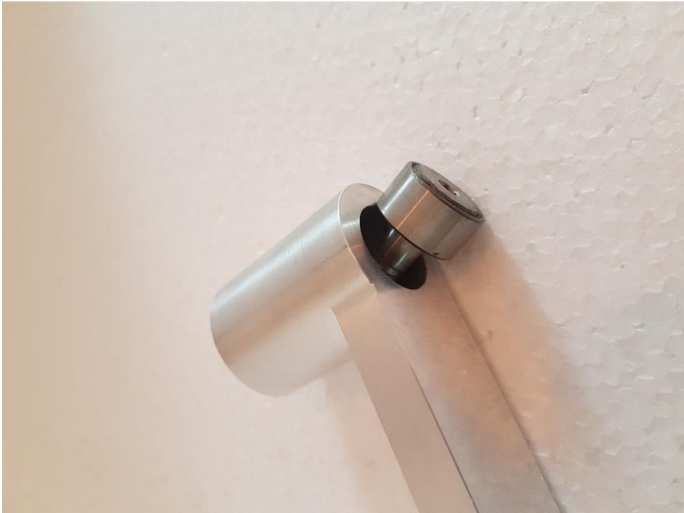
Figure 2.17. Type 2 bearing sliding into primary arm
