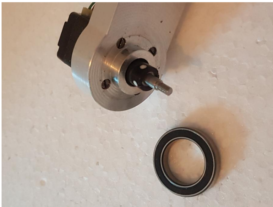
Figure 2.20. Type 1 bearing that slips on under actuator
