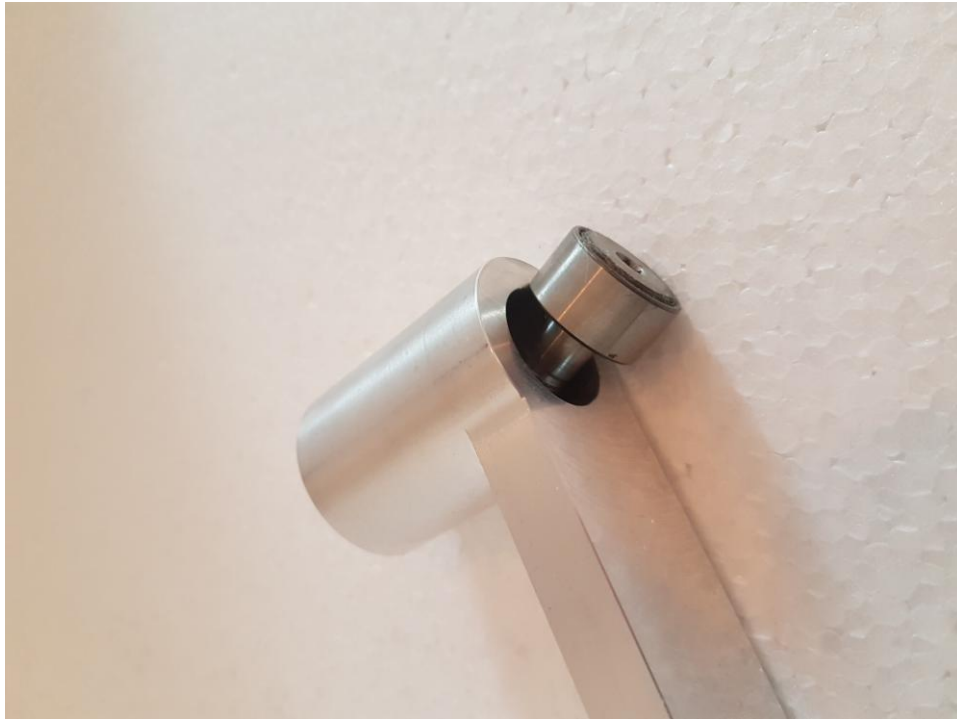
Figure 2.17. Type 2 bearing sliding into primary arm
