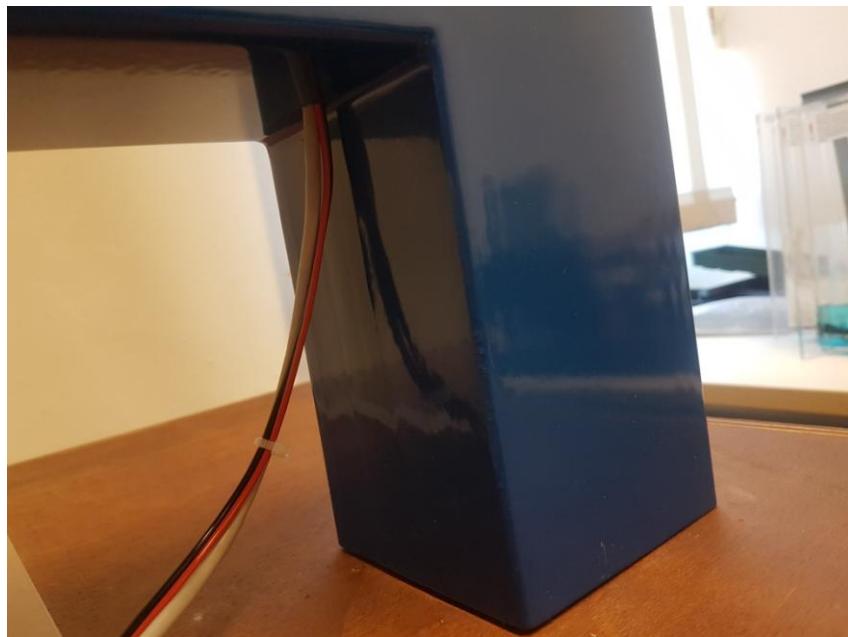
Figure 3.5. Hole for wires from actuator and solenoid
