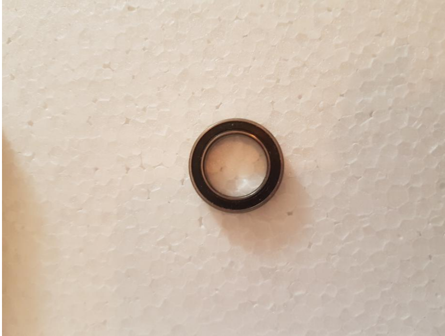
Figure 2.12. Bearing type 1 for end of arm connection
