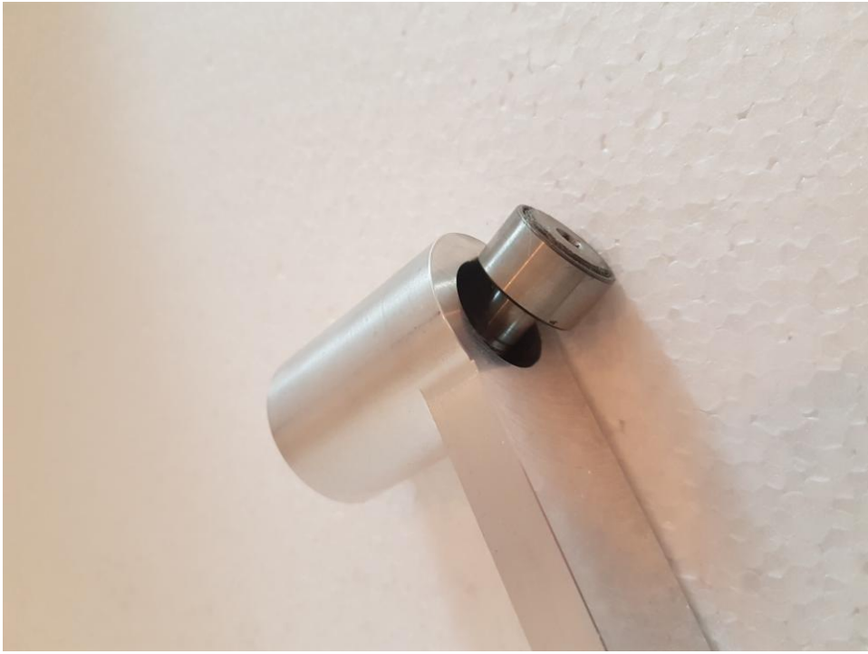
Figure 2.17. Type 2 bearing sliding into primary arm
