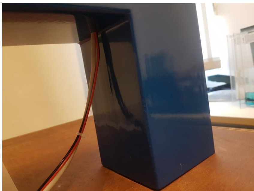
Figure 3.5. Hole for wires from actuator and solenoid
